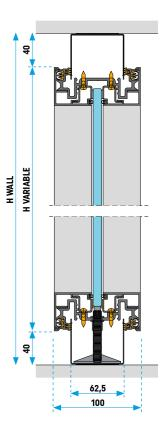
The **DUO** partition system is made of seamless glass panels, single or double, framed in aluminum and steel structure, self-bearing, with independent construction components, and is fitted with polycarbonate sealing joints. These walls secure an excellent acoustic performance and ensure clear-cut aesthetics, with the vertical and horizontal profiles on the perimeter connections.
