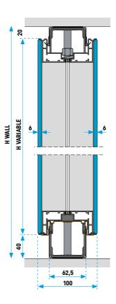
LUCE Partitions is a system of mobile walls with internal steel-framed structure fitted with solid or glass panels, featuring an exclusive patented system to fit the panels and glass frames with a snap-on action that eliminates
