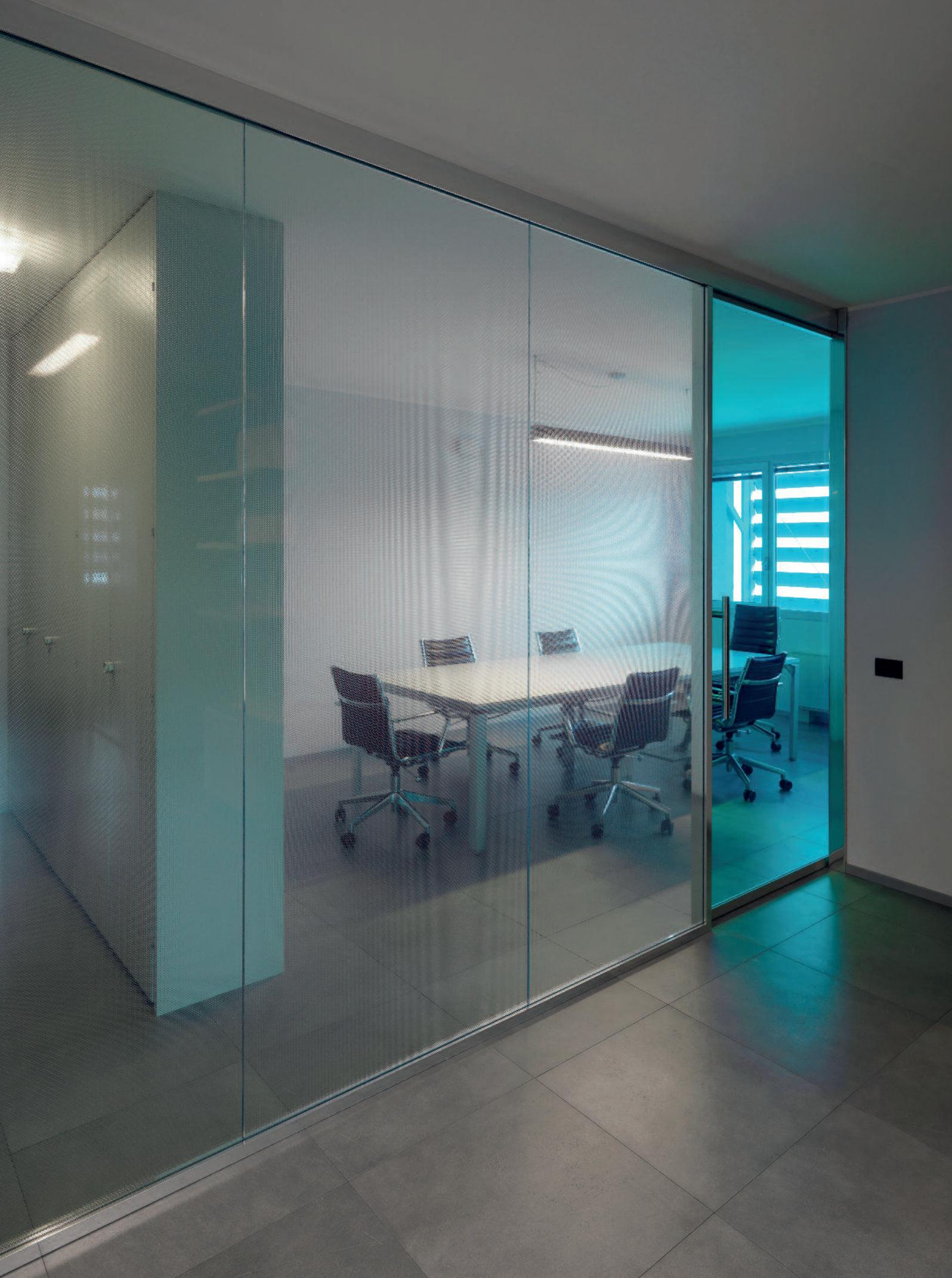
**NEXUS** partition system is made of single seamless glass panels, framed in aluminum structure, self-bearing, with independent construction components, fitted with polycarbonate sealing joints. These walls secure a good acoustic performance and provide a satisfactory clear-cut aesthetics, with the vertical and horizontal profiles on the perimeter connections.
