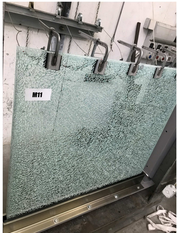
Photograph of the railing after breakage
