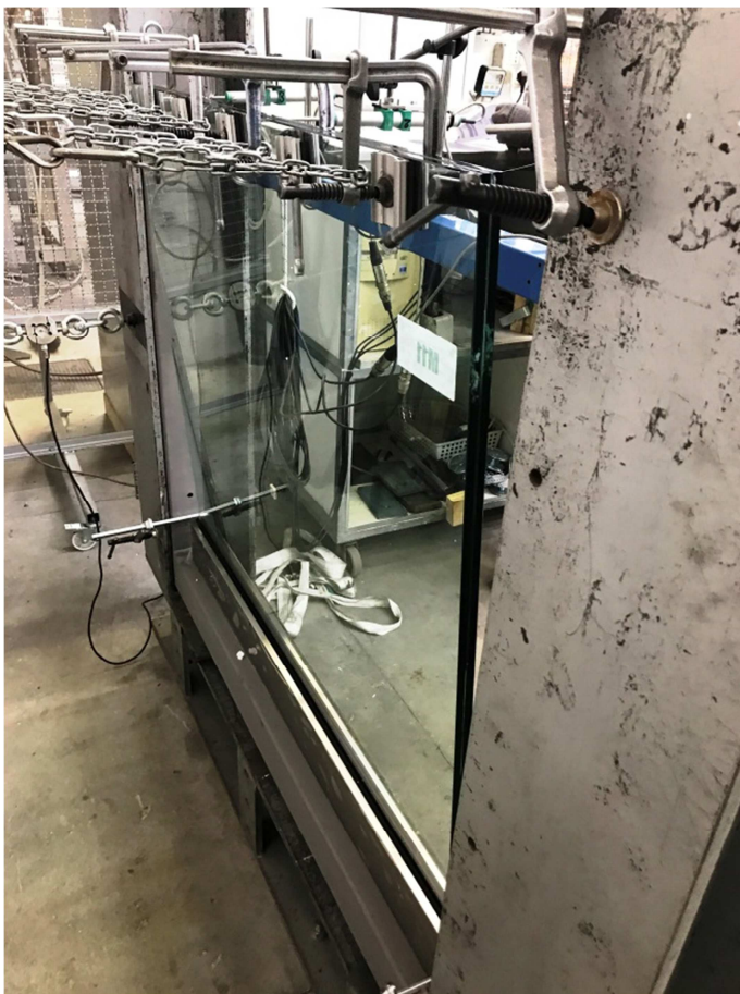
Photograph of the railing subjected to working load
