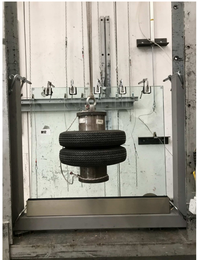
Photograph of the railing after double-tire body impact
