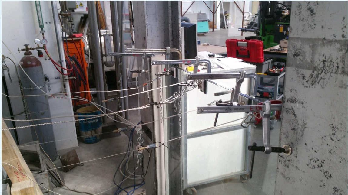
Photograph of the sample during outward horizontal static loading test
